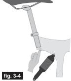
which is to make it easy to see whether the seatpost is inserted in the seat tube far enough to be safe. If your bicycle has such a sight hole, use it instead of the "Minimum Insertion" or "Maximum Extension" mark to 20 Fit Saddle position
